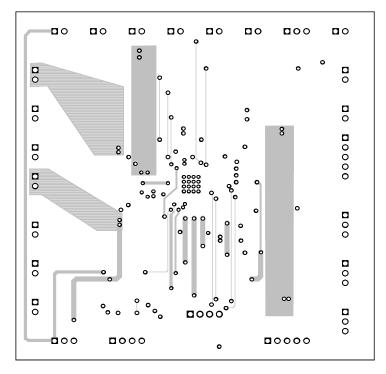
Figure 3-5. Bottom Layer Routing
