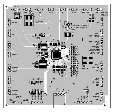
Figure 3-2. Top Layer Routing
