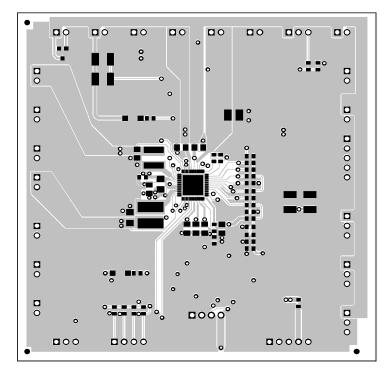
Figure 3-3. Layer 2 Routing
